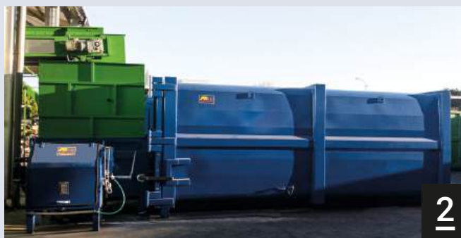
1. Two independent chambers compactor Compactor cu două camere independente
