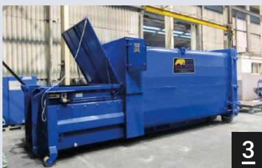
1. Two independent chambers compactor Compactor cu două camere independente
